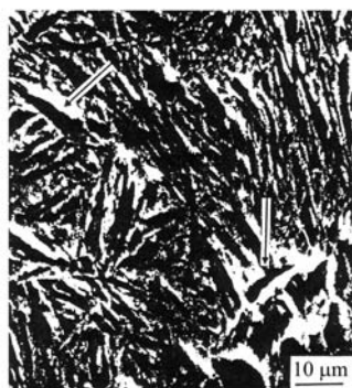
Fig. 3 SEM micrograph of low alloy Cr–Mo steel after quenching at a rate of 30 K s -1 . Arrows point to martensite laths
