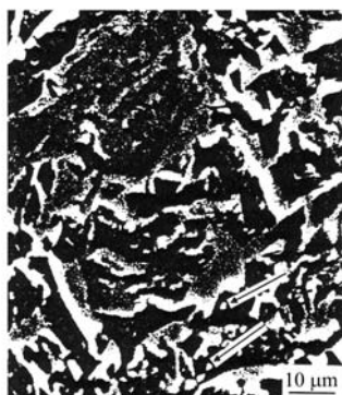
Fig. 1 SEM micrograph of low alloy Cr–Mo steel after hot rolling. Arrows point to carbide particles
