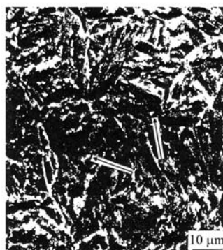
Fig. 4 SEM micrograph of low alloy Cr–Mo steel after tempering at 823 K for 360 s. Arrows point to carbide particles
